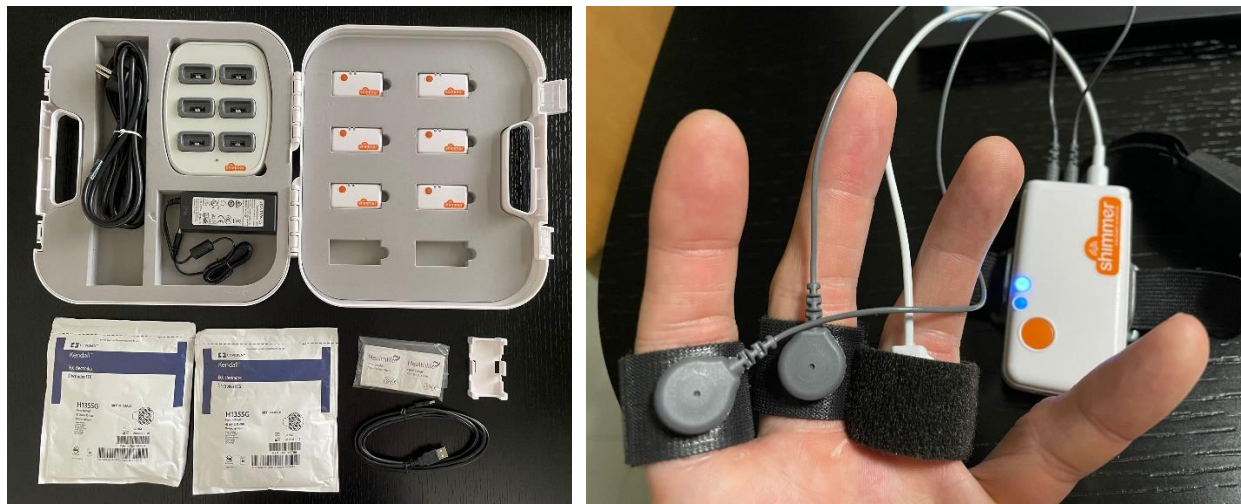
Figure 4. Biosensors to capture sympathetic nervous system responses including skin conductance, heart rate and heart rate variability.
